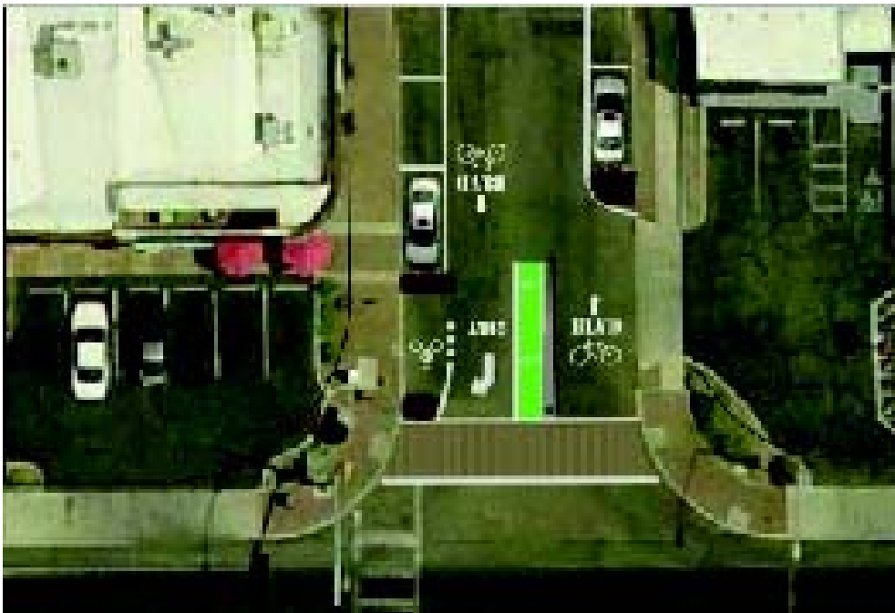
A similar TOUCAN style upgrade is proposed for the Treat Avenue and Speedway Boulevard crossing to make the intersection safer and more appealing to users.
