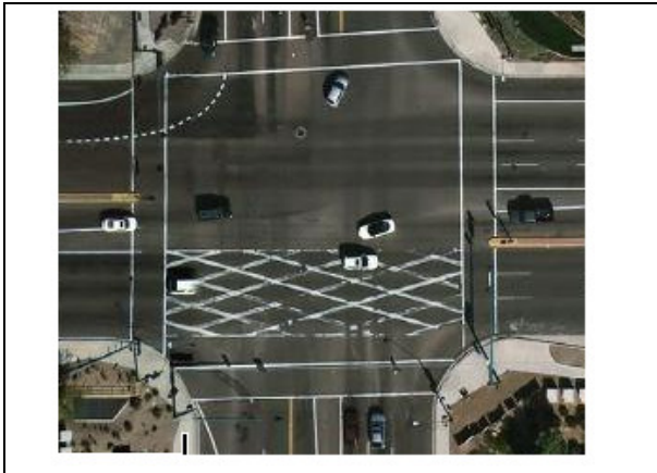
Figure 10: Pavement markings and signing to discourage blocking of intersection by vehicles
